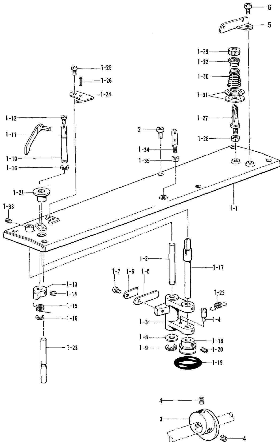
K. 糸巻き関係 / Bobbin winder mechanism / Spuler /
